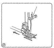
3 Pull both threads under and to the back of the presser foot, leaving 4 to 6 inches of thread clear.
